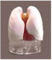
The set of RI container inserts can be set in the chest phantom in place of standard inserts allowing wider research applications including PET/CT fusion evaluation.
